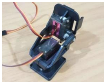
Figure 2. MG90S micro servo on 2 axis camera gimbals
