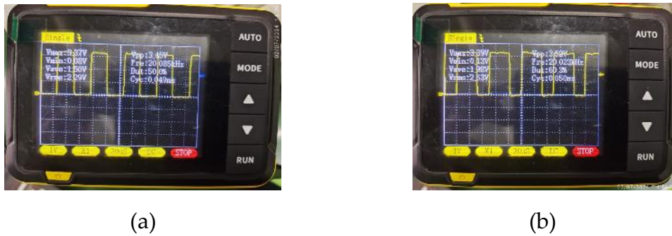
Figure 8. (a) PWM Output Testing Results Pin 18, (b) PWM Pin 19 Output Testing Results
