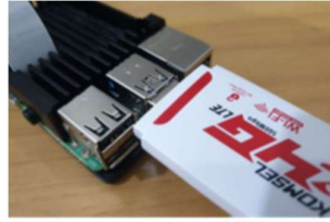
Figure 3. Raspberry Pi 4 USB port connected to LTE Wi-Fi dongle
