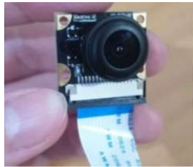
Figure 1. OV5647 camera module
