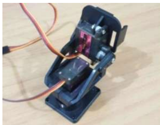
Figure 2. MG90S micro servo on 2 axis camera gimbals
