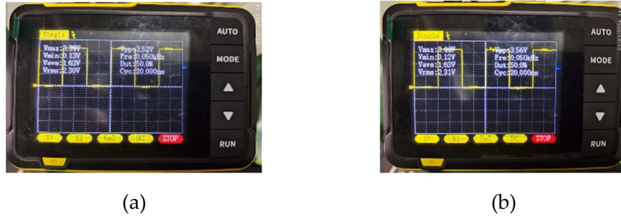
Figure 7. (a) PWM Pin 27 Output Testing Results, (b) PWM Pin 26 Output Testing Results
