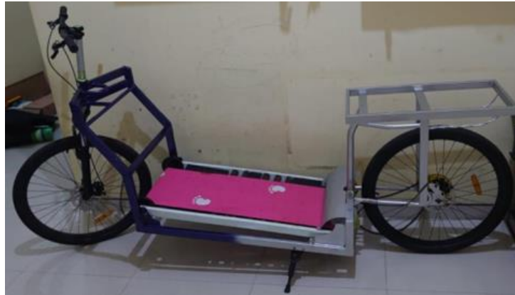
Gambar 6. Hasil Rancang Bangun Sepeda Treadmill
